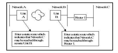
To continue with this example, if Network B is not configured to advertise Network C to Network A, then Network A will not dynamically learn of Network C's existence. If you wish to establish a route on Network A to Network C, you must define a static route on Network A that indicates that Network C may be accessed through remote Adit B.
